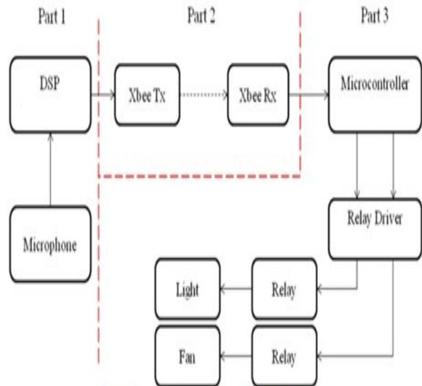
Fig 1: Proposed block diagram of the Smart Home Control System
