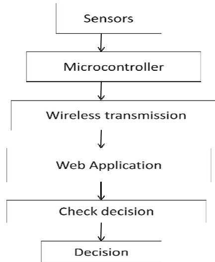
Figure 1: Block Diagram of wearable health Monitoring
