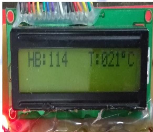
Figure 3: Digital output displayed on LCD
