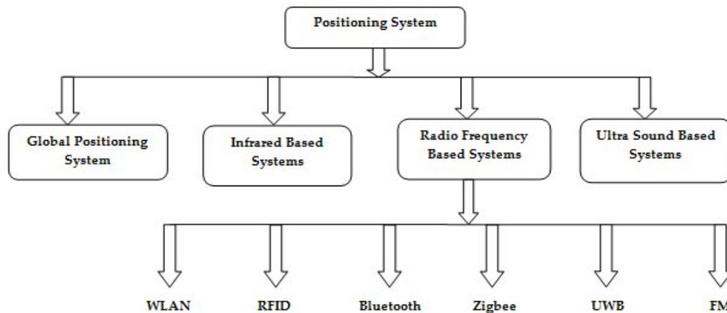
Figure 4: Wireless Positioning Technologies
